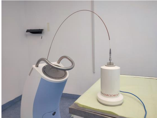
Figure 1. The after-loading unit and well-type ion chamber
