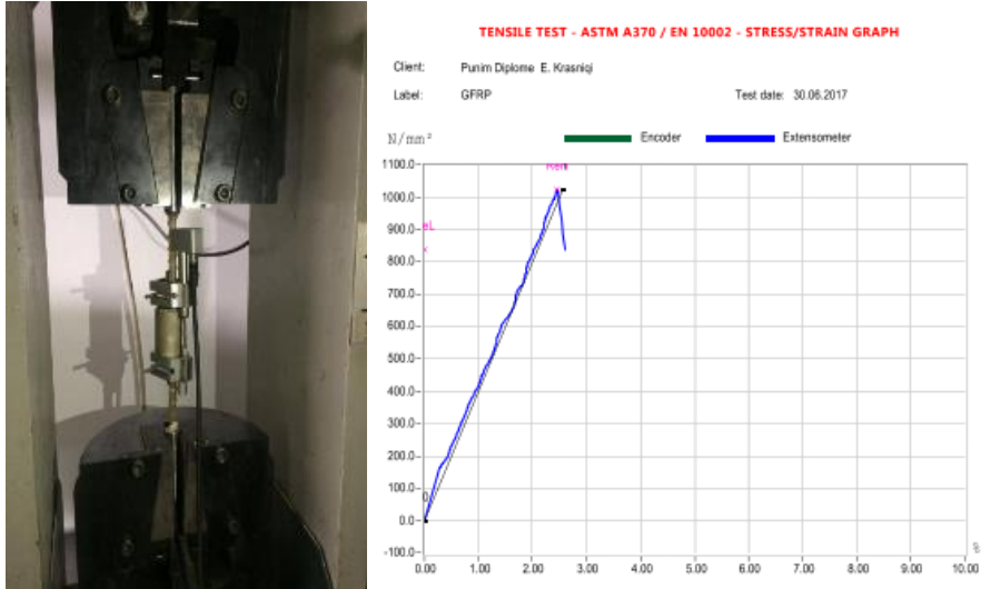
Fig. 12. Examinations of mechanical properties of GFRP bars
