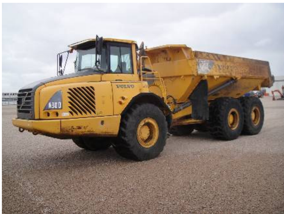
Fig.83) Kamioni transportues Damper, Volvo model A30D, 440KS.
